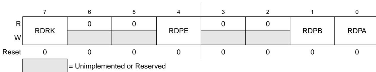
Figure 21-15. Reduced Drive Register (RDRIV)
