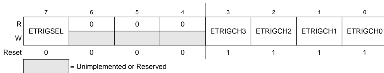
Figure 7-4. ATD Control Register 1 (ATDCTL1)
