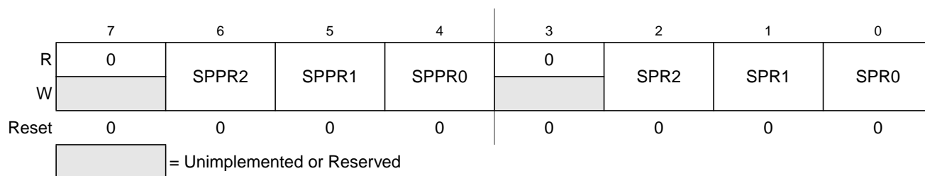
Figure 14-5. SPI Baud Rate Register (SPIBR)
