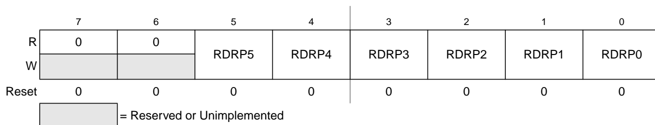
Figure 4-26. Port P Reduced Drive Register (RDRP)
