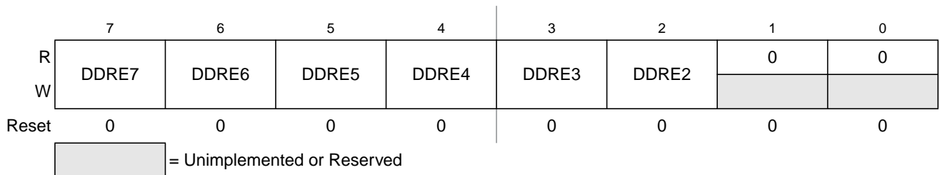
Figure 24-8. Port E Data Direction Register (DDRE)
