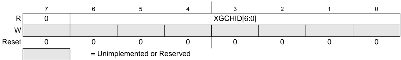
Figure 6-4. XGATE Channel ID Register (XGCHID)
