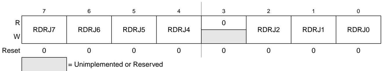
Figure 23-59. Port J Reduced Drive Register (RDRJ)
