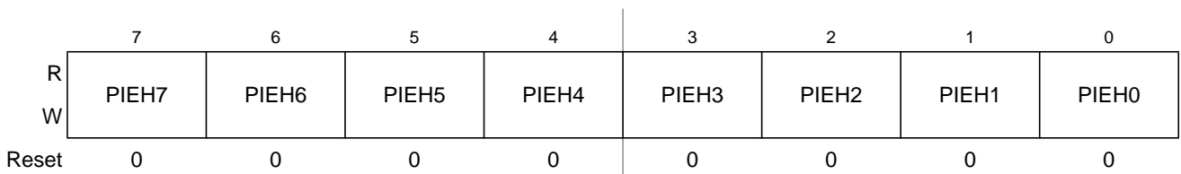
Figure 23-54. Port H Interrupt Enable Register (PIEH)
