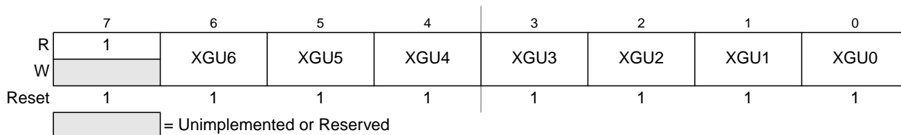
Figure 25-18. RAM XGATE Upper Boundary Register (RAMXGU)
