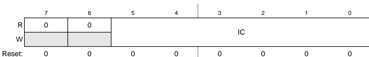
Figure 24-3. I 2 C Frequency Divider Register (I2FDR)
