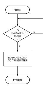
Figure 14-27. UART Mode Programming Flowchart (Sheet 5 of 5)
