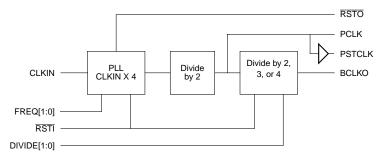
Figure 7-1. PLL Module Block Diagram
