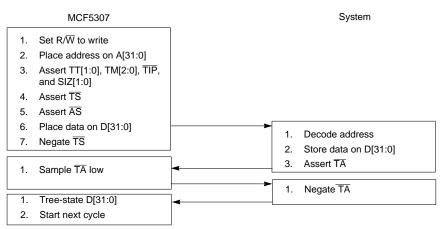
Figure 18-7. Write Cycle Flowchart
