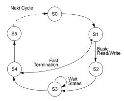
Figure 18-4. Data Transfer State Transition Diagram
