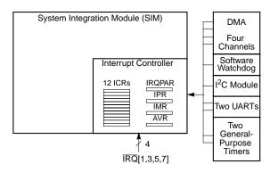
Figure 9-1. Interrupt Controller Block Diagram
