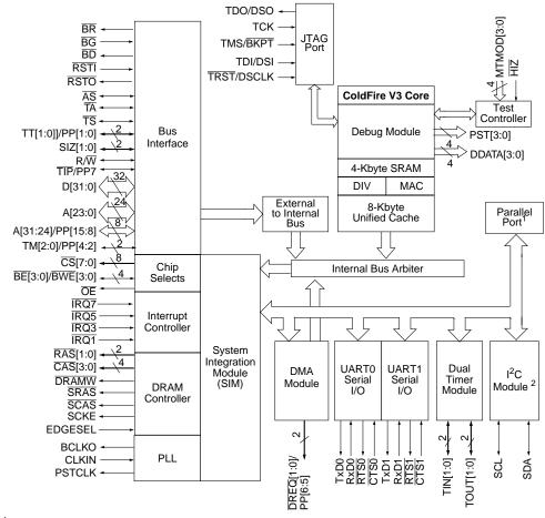
$^1$  Note: Parallel port pins (PPn) are multiplexed with other bus functions as shown.  $^2$   $^1{}^2C$  is a Philips proprietary interface
