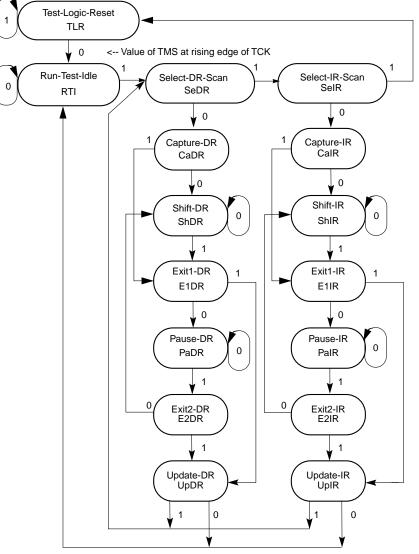
Figure 19-2. JTAG TAP Controller State Machine
