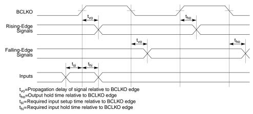
Figure 18-1. Signal Relationship to BCLKO for Non-DRAM Access
