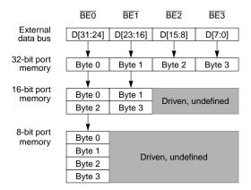
Figure 10-1. Connections for External Memory Port Sizes
