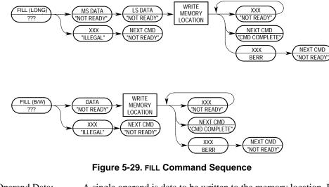
Operand Data:A single operand is data to be written to the memory location. Byte<br/>data is sent as a 16-bit word, justified in the least-significant byte; 16-<br/>and 32-bit operands are sent as 16 and 32 bits, respectively.Result Data:Command complete status (0xFFFF) is returned when the register<br/>write is complete. A value of 0x0001 (with S set) is returned if a bus<br/>error occurs.
