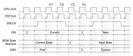
Figure 5-13. BDM Serial Interface Timing
