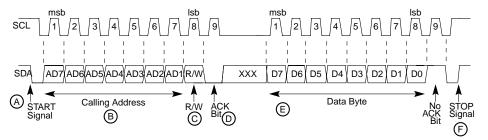
Figure 8-2. I<sup>2</sup>C Standard Communication Protocol
