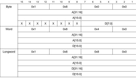
Figure 5-24. WRITE Command Format
