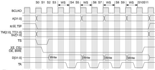
Figure 18-17 shows a line burst write with one wait-state insertion.
