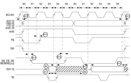
Figure 20-3. AC Timings—Normal Read and Write Bus Cycles
