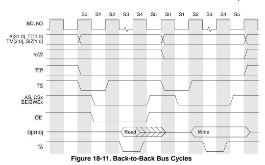
Basic read and write cycles are used to show a back-to-back cycle, but there is no restriction as to the type of operations to be placed back to back. The initiation of a back-to-back cycle is not user definable.
