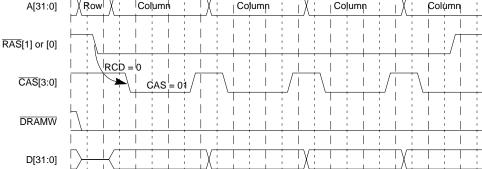
Figure 11-8. Burst Page-Mode Write Operation (4-3-3-3)
