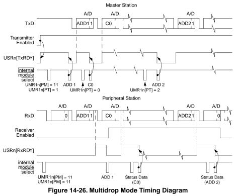
A character sent from the master station consists of a start bit, a programmed number of data bits, an address/data (A/D) bit flag, and a programmed number of stop bits. A/D = 1 indicates an address character; A/D = 0 indicates a data character. The polarity of A/D is selected through UMR1*n*[PT]. UMR1*n* should be programmed before enabling the
