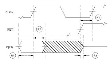
Note: Mode selects are registered on the rising CLKIN edge before the cycle in which RSTI is recognized as being negated.
