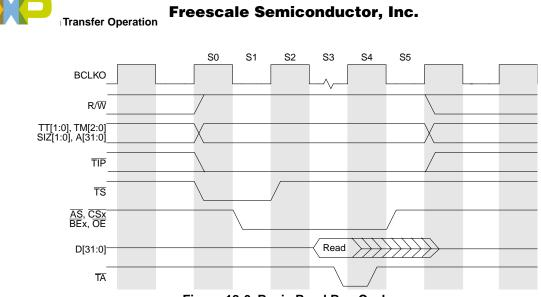
Figure 18-6. Basic Read Bus Cycle
