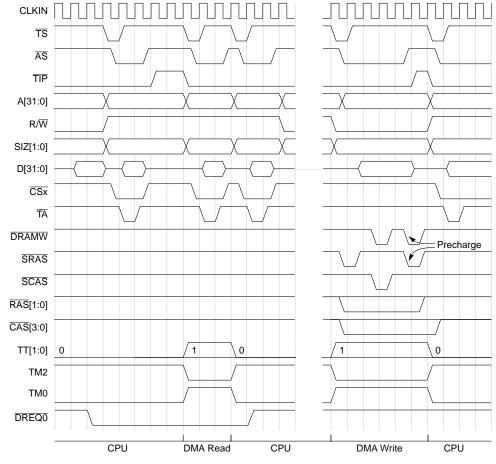
Figure 12-12. Dual-Address, Peripheral-to-SDRAM, Lower-Priority DMA Transfer
