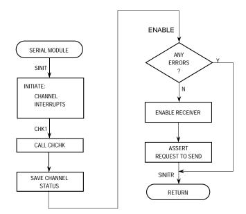
Figure 14-27. UART Mode Programming Flowchart (Sheet 1 of 5)
