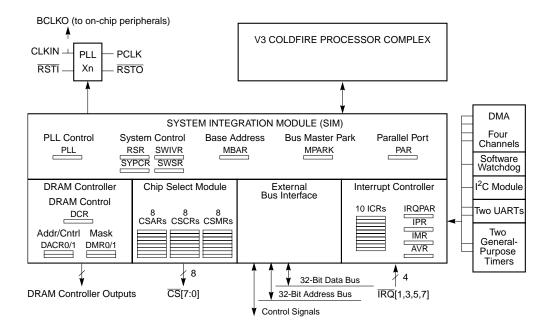
Figure 6-1. SIM Block Diagram
