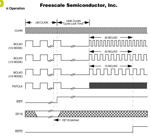
Figure 18-34. Software Watchdog Reset Timing
