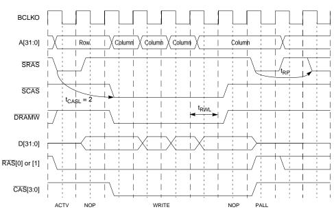
Figure 11-19. Burst Write SDRAM Access
