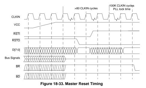
During the master reset period, all signals capable of being three-stated are driven to a high-impedance; all others are negated. When  $\overline{RSTI}$  negates, all bus signals remain in a high-impedance state until the MCF5307 is granted the bus and the core begins the first bus cycle for reset exception processing. A master reset causes any bus cycle (including DRAM refresh cycle) to terminate and initializes registers appropriately for a reset exception.
