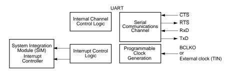
Figure 14-1. Simplified Block Diagram
