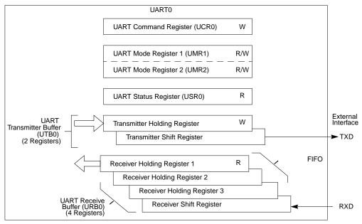
Figure 14-20. Transmitter and Receiver Functional Diagram
