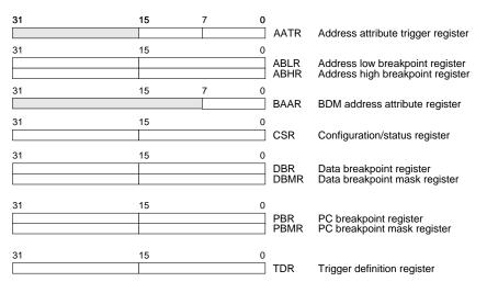
Note: Each debug register is accessed as a 32-bit register; shaded fields above are not used (don't care). All debug control registers are writable from the external development system or the CPU via the WDEBUG instruction.
