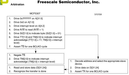
Figure 18-23. Interrupt-Acknowledge Cycle Flowchart
