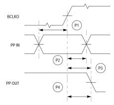
Figure 20-17. General-Purpose I/O Timing
