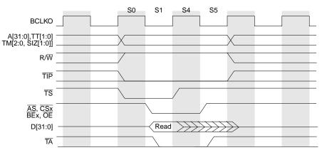
Figure 18-9. Read Cycle with Fast Termination
