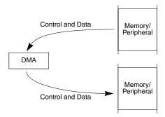
Figure 12-2. Dual-Address Transfer
