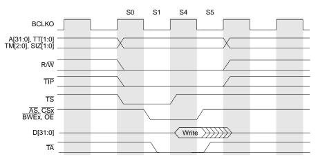
Figure 18-10. Write Cycle with Fast Termination
