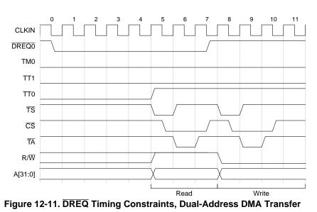
Although Figure 12-11 does not show TM0 signaling a DMA acknowledgement, this signal can provide an external request acknowledge response, as shown in subsequent diagrams.
