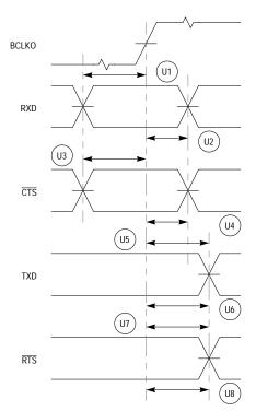
Figure 20-16. UART0/1 Module AC Timing—UART Mode
