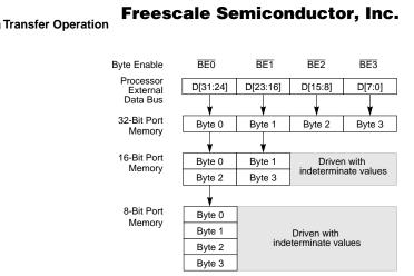
Figure 18-2. Connections for External Memory Port Sizes
