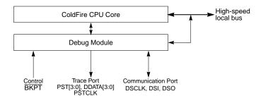
Figure 5-1. Processor/Debug Module Interface
