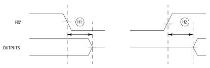
Figure 20-10. AC Output Timing—High Impedance
