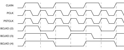
NOTE: The clock signals are shown with edges aligned to show frequency relationships only. Actual signal edges have some skew between them.
