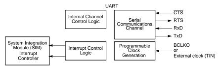
Figure 1-2. UART Module Block Diagram
