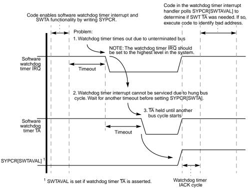
Figure 6-4. MCF5307 Embedded System Recovery from Unterminated Access
