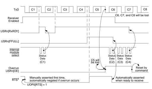
Figure 14-22. Receiver Timing
