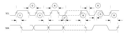
Figure 20-15. I<sup>2</sup>C Input/Output Timings
