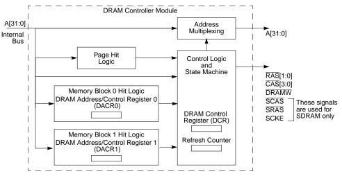
Figure 11-1. Asynchronous/Synchronous DRAM Controller Block Diagram
