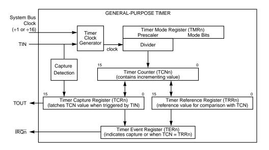
Figure 13-1. Timer Block Diagram
