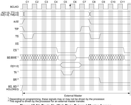
Figure 18-24. Basic No-Wait-State External Master Access
