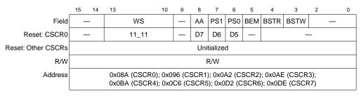
Figure 10-4. Chip-Select Control Registers (CSCR0–CSCR7)
