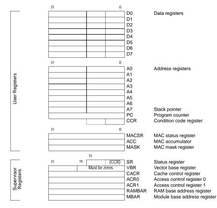
Figure 1-4. ColdFire MCF5307 Programming Model
