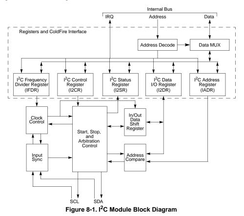
Figure 8-1 shows the relationships of the I<sup>2</sup>C registers, listed below:
