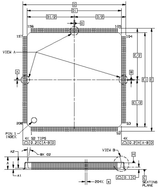
Figure 16-2. MCF5307 Case Drawing (General View)
