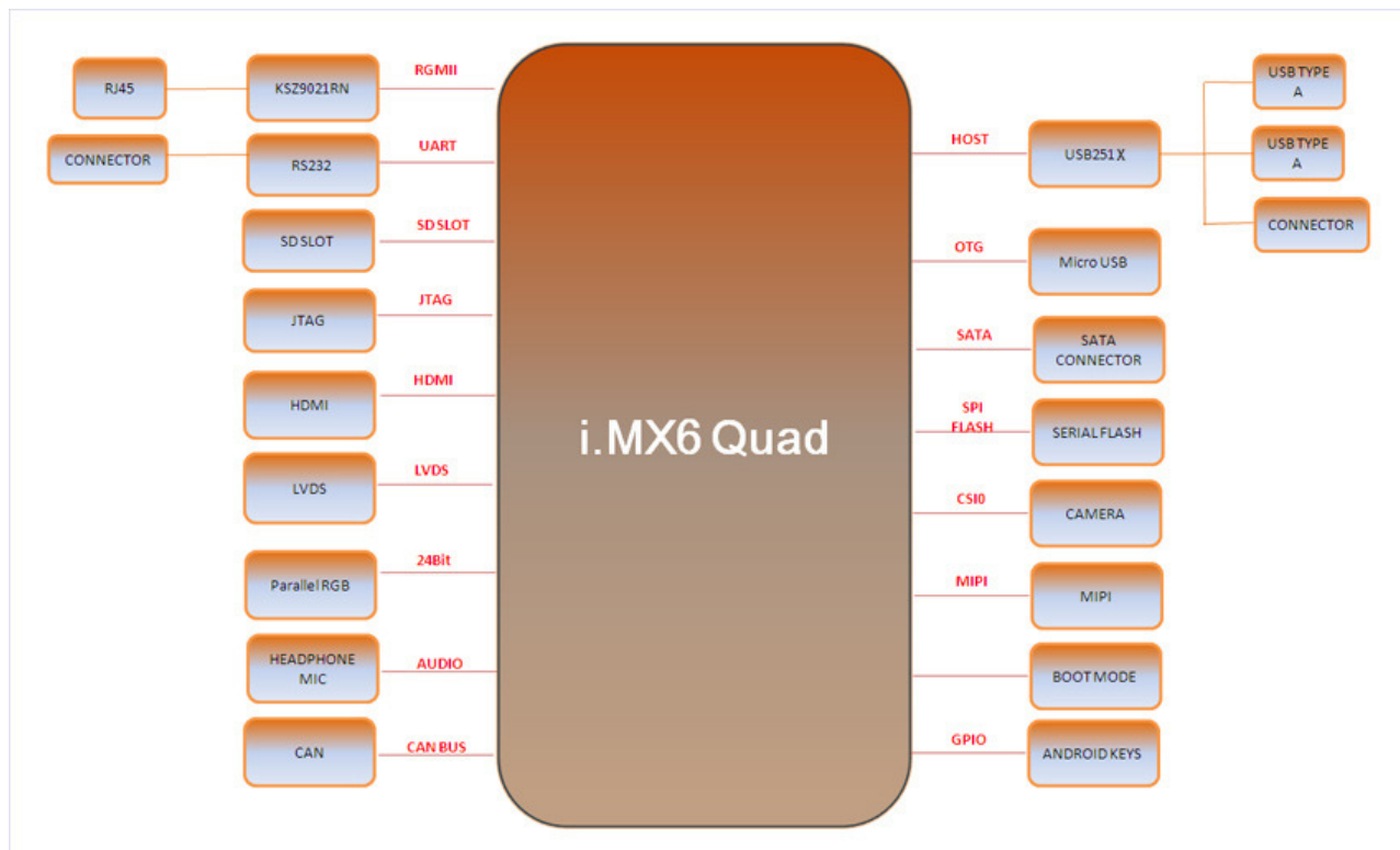
Figure 1 Functional Block Diagram of SABRE Lite Board
