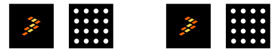
80 WLCSP (AP) 80 WLCSP (BP) 4.13 x 3.56 x 0.564 mm 4.13 x 3.56 x 0.321 mm Pitch 0.4 mm Pitch 0.4 mm
