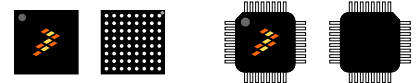
144 MABGA (MD) 13 mm x 13 mm Pitch 1 mm 144 LQFP (LQ) 20 mm x 20 mm Pitch 0.5 mm
