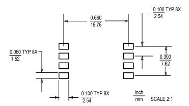
Figure 9. SOP footprint (case 98ASB17757C)
