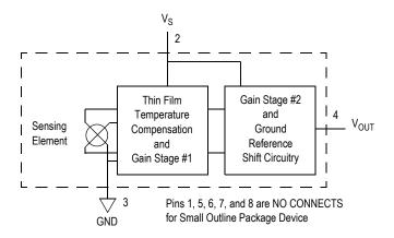
Figure 1. Fully integrated pressure sensor block diagram
