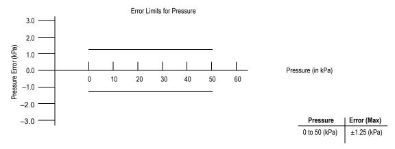
Figure 8. Pressure error band
