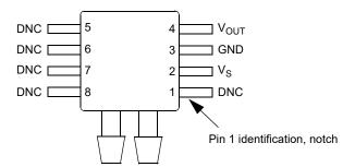
Figure 2. Device pinout (top view)
