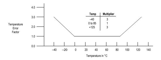
NOTE: The Temperature Multiplier is a linear response from 0  $^{\circ}$ C to -40  $^{\circ}$ C and from 85  $^{\circ}$ C to 125  $^{\circ}$ C.
