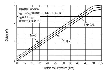
Figure 3. Output versus Pressure differential
