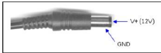
Figure 3: 2.1 mm Power Connector
