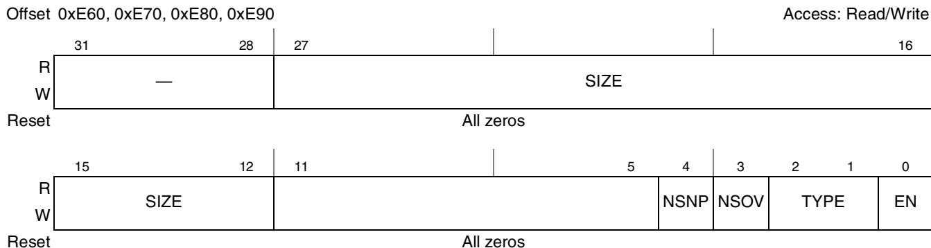
Figure 15-135. PCI Express RC Inbound Window Attributes Register n (PEX_RCIWAR0–PEX_RCIWAR3)
