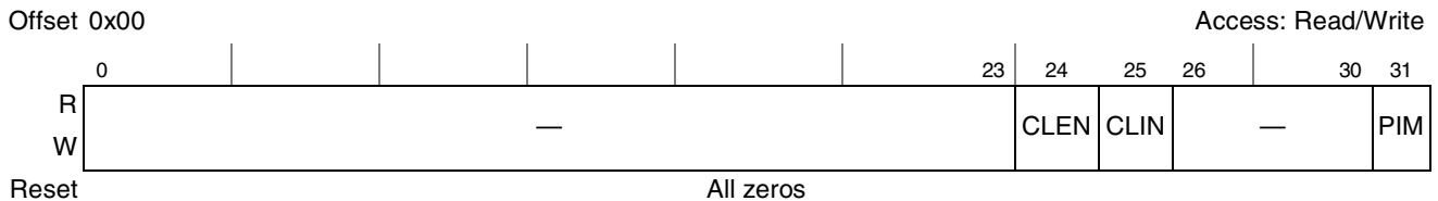
Figure 5-39. Periodic Interval Timer Control Register (PTCNR)
