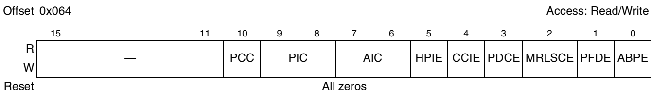
Figure 15-58. PCI Express Slot Control Register
