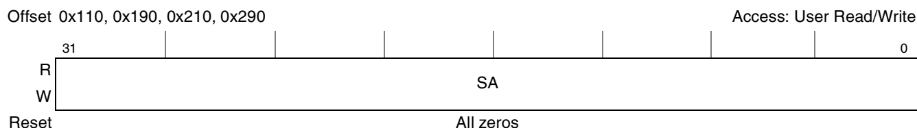
Figure 13-13. DMA Source Address Register (DMASAR n )
