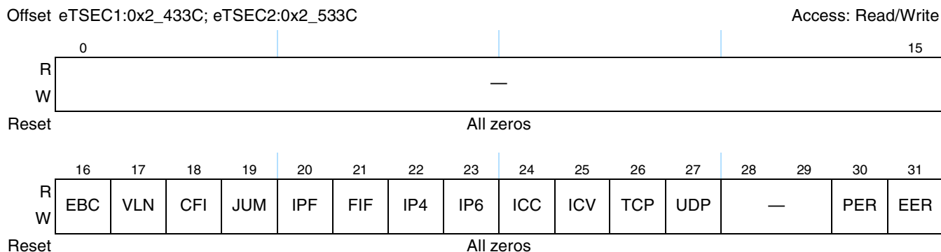
Figure 18-30. Receive Queue Filer Table Property ID1 Register Definition
