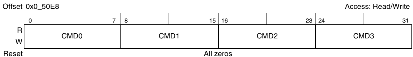
Figure 10-22. Flash Command Register
