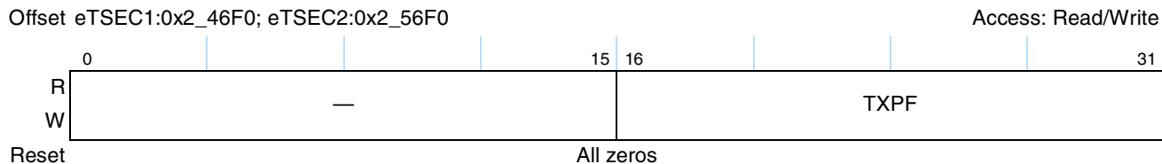
Figure 18-79. Transmit Pause Control Frame Counter Register Definition
