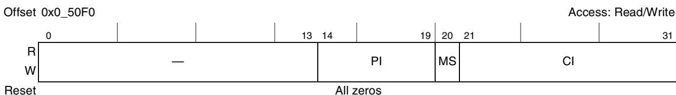
Figure 10-25. Flash Page Address Register, Large Page Device (OR \eta [PGS] = 1)
