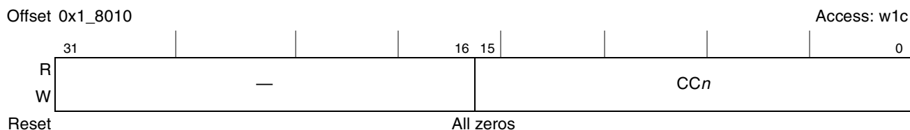
Figure 16-4. Command Completed Register (CCR)
