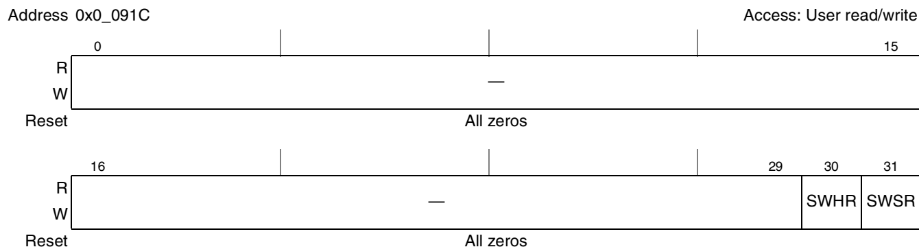
Figure 4-12. Reset Control Register (RCR)
