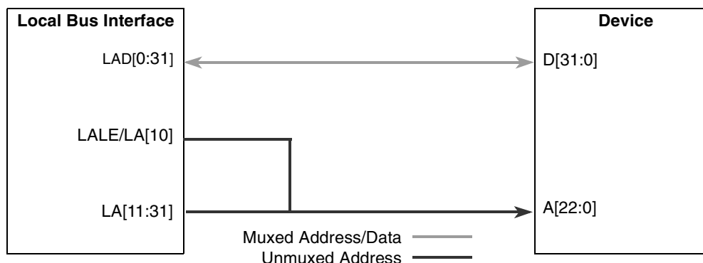
Figure 10-71. Non-Multiplexed Address and Data Buses
