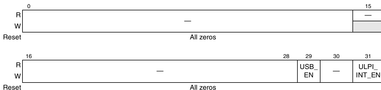
Figure 20-34. USB General-Purpose Register (CONTROL)
