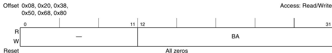
Figure 12-3. PCI Outbound Base Address Registers (POBAR n )
