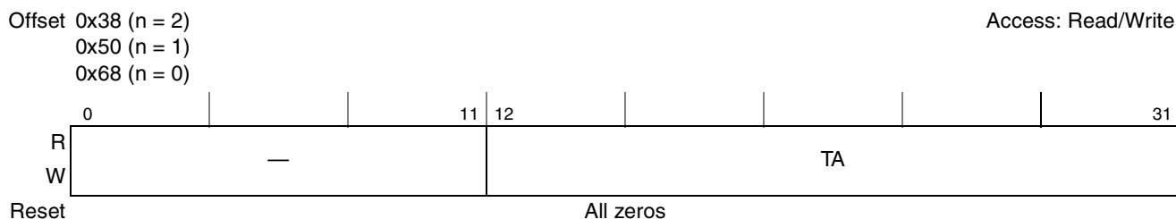
Figure 14-15. PCI Inbound Translation Address Registers (PITAR n )
