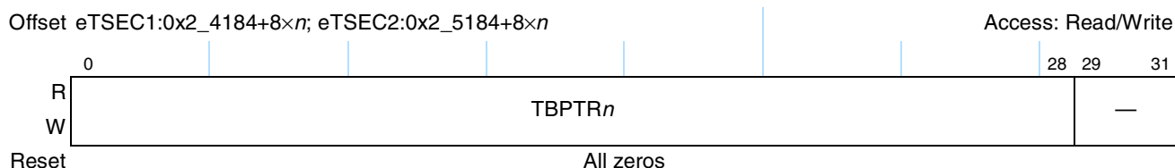
Figure 18-18. TBPTR0–TBPTR7 Register Definition
