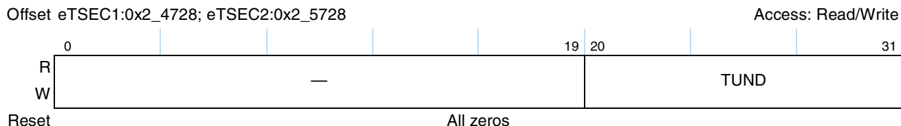
Figure 18-92. Transmit Undersize Frame Counter Register Definition
