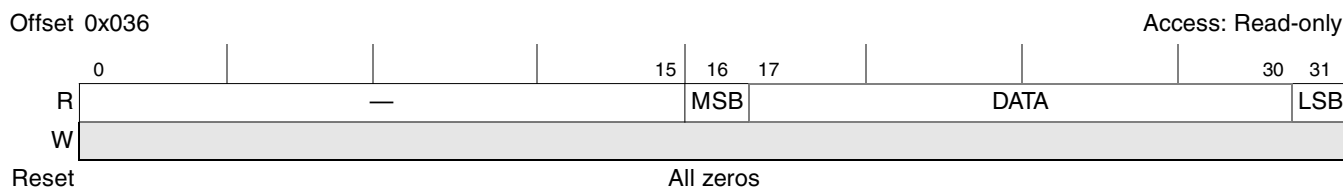
Figure 23-14. Example SPMode[REV] = 1 SPMode[LEN] = 15 MSB Sent First
