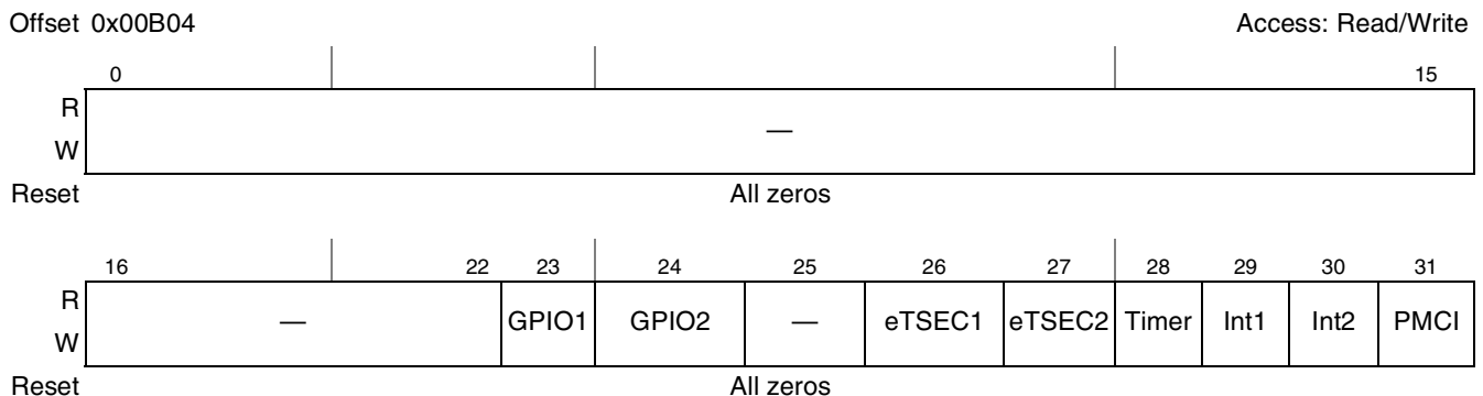
Figure 5-58. Power Management Controller Event Register
