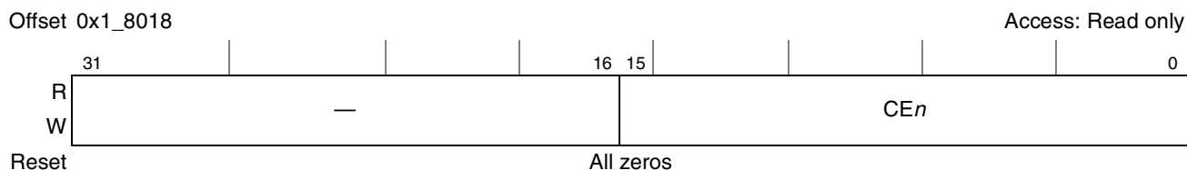
Figure 16-5. Command Error Register (CER)
