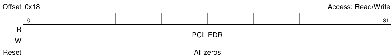
Figure 14-11. PCI Error Data Low Capture Register (PCI_EDLCR)
