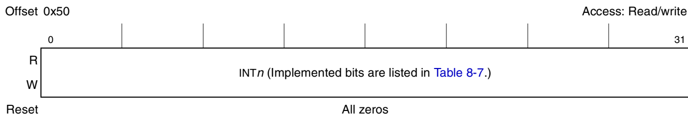
Figure 8-22. System Internal Interrupt Force Register (SIFCR_H)
