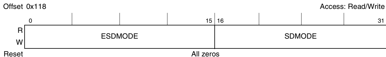
Figure 9-10. DDR SDRAM Mode Configuration Register (DDR_SDRAM_MODE)
