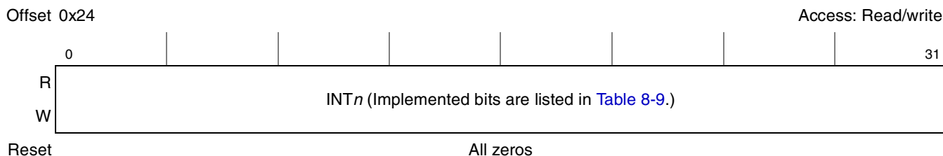
Figure 8-11. System Internal Interrupt Mask Register (SIMSR_L)
