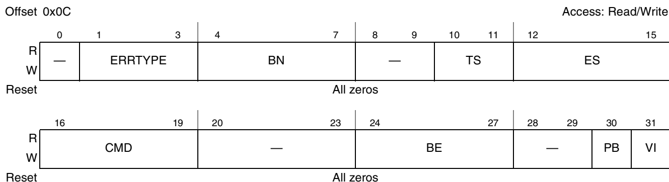
Figure 14-8. PCI Error Attributes Capture Register (PCI_EATCR)
