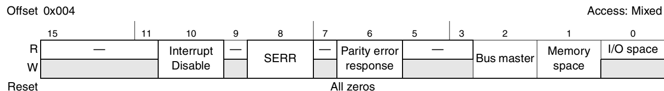
Figure 15-5. PCI Express Command Register
