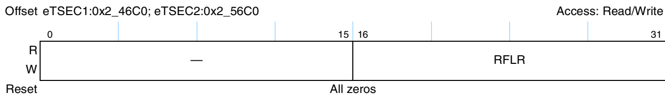
Figure 18-67. Receive Frame Length Error Counter Register Definition
