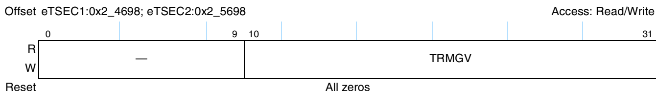
Figure 18-57. Transmit and Received 1519- to 1522-Byte VLAN Frame Register Definition
