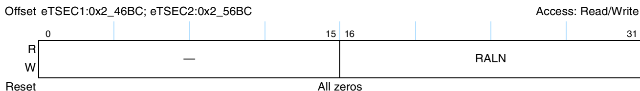
Figure 18-66. Receive Alignment Error Counter Register Definition
