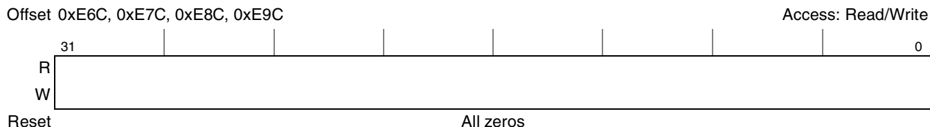
Figure 15-138. CI Express RC Inbound Window Base Address Register High n (PEX_RCIWBARH0–PEX_RCIWBARH3)
