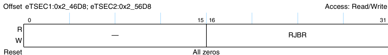
Figure 18-73. Receive Jabber Counter Register Definition
