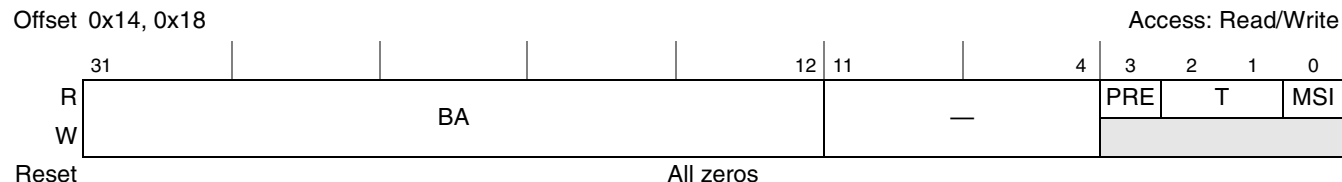
Figure 14-32. GPL Base Address Register 0
