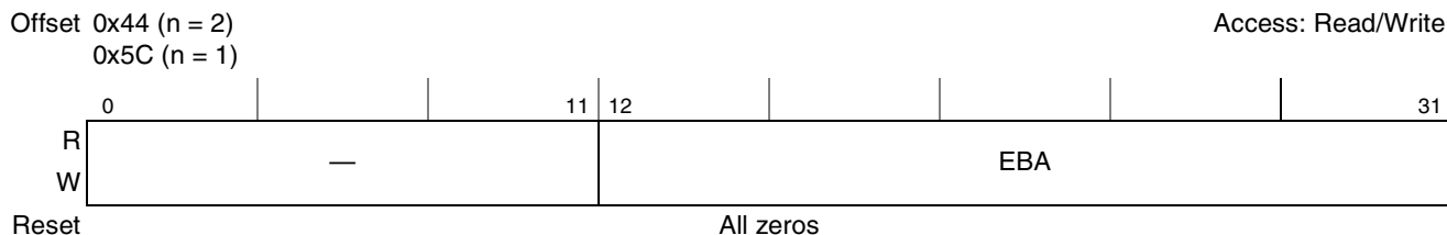
Figure 14-17. PCI Inbound Extended Base Address Registers (PIEBAR n )
