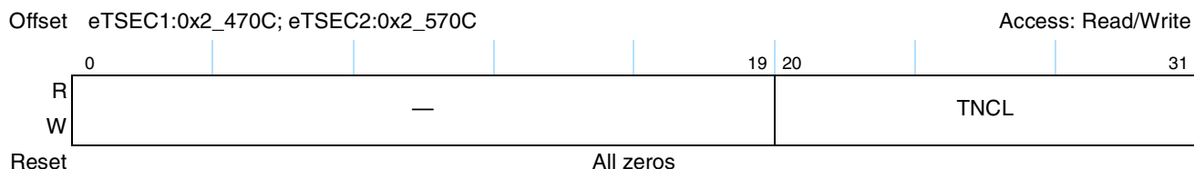
Figure 18-86. Transmit Total Collision Counter Register Definition
