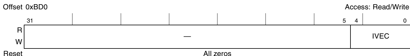
Figure 15-119. PCI Express Host Read DMA Interrupt Vector Register (PEX_HRDIVR)
