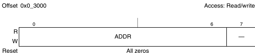
Figure 21-2. I 2 C n Address Register (I2C n ADR)
