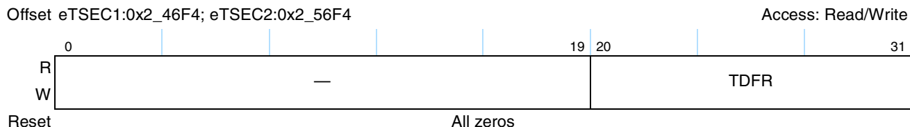
Figure 18-80. Transmit Deferral Packet Counter Register Definition
