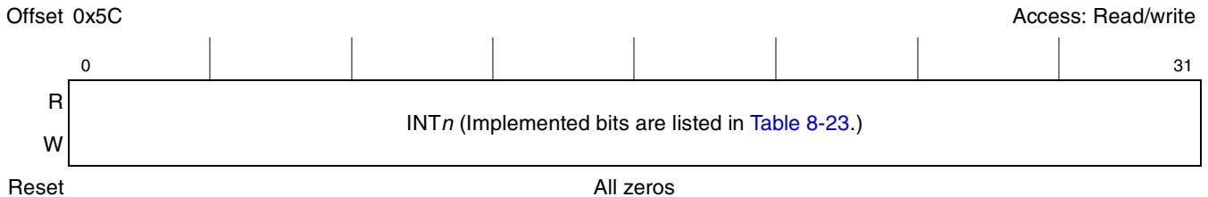
Figure 8-25. System Error Status Register (SERFR)
