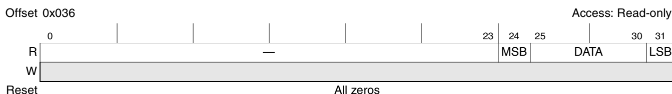
Figure 23-13. Example SPMODE[REV] = 1 SPMODE[LEN] = 7 MSB Sent First
