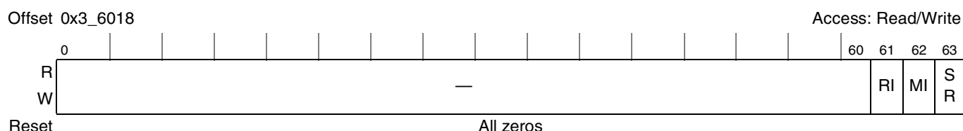
Figure 17-85. MDEU Reset Control Register
