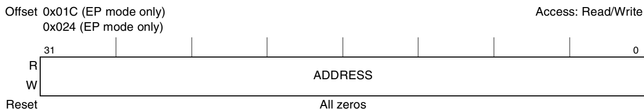
Figure 15-15. 64-Bit High Memory Base Address Registers 3 and 5 (BAR3/BAR5)
