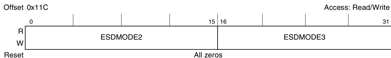
Figure 9-11. DDR SDRAM Mode 2 Configuration Register (DDR_SDRAM_MODE_2)
