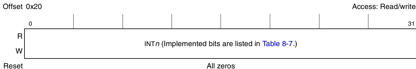
Figure 8-10. System Internal Interrupt Mask Register (SIMSR_H)
