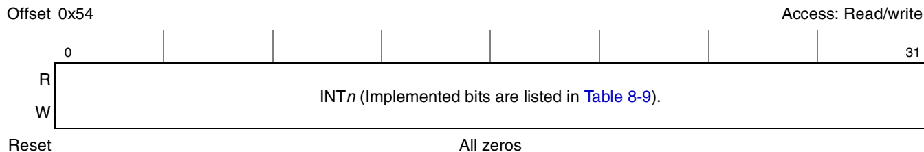
Figure 8-23. System Internal Interrupt Force Register (SIFCR_L)
