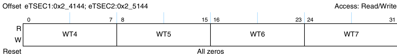
Figure 18-17. TR47WT Register Definition
