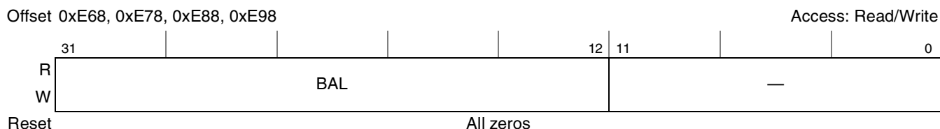
Figure 15-137. PCI Express RC Inbound Window Base Address Register Low n (PEX_RCIWBARL0–PEX_RCIWBARL3)
