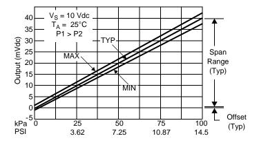
Figure 3. Output versus Pressure Differential
