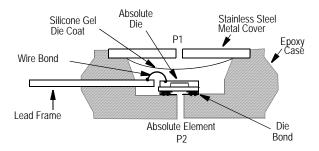
Figure 4. Cross-Sectional Diagram (not to scale)
