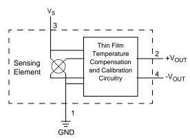
Figure 1. Temperature Compensated Pressure Sensor Schematic
