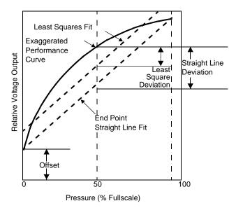
Figure 2. Linearity Specification Comparison
