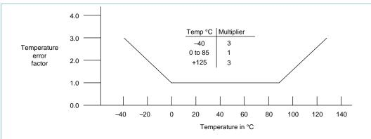
Note: The temperature multiplier is a linear response from 0°C to -40°C and from 85°C to 125°C.
