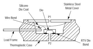
Figure 3. Cross-Sectional Diagrams (not to scale)
