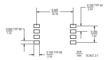
Figure 7. SOP footprint (case 98ASB17756C)
