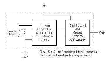
Figure 1. Integrated pressure sensor schematic
