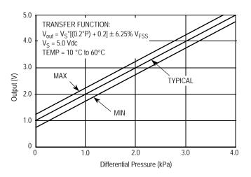
Figure 5. Output vs. pressure differential at ±6.25% V<sub>FSS</sub> (without autozero, Table 3, note 5)
