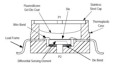
Figure 3. Cross-sectional diagram (not to scale)
