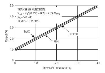
Figure 6. Output vs. pressure differential at ±2.5% V<sub>FSS</sub> (with autozero, Table 3, note 5)
