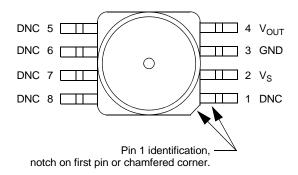
Figure 2. Device pinout (top view)
