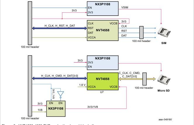
Figure 2. NVT4558-4858-EVB evaluation board block diagram
