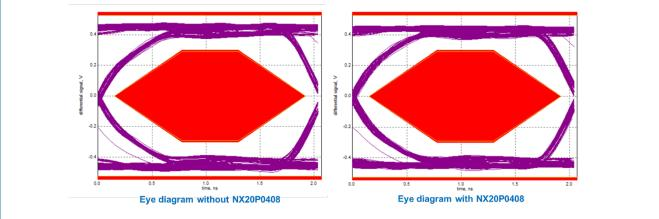
Figure 7. USB high speed eye diagram of USB switch
