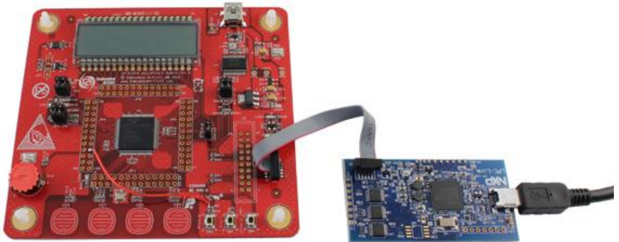
Figure 7 – LPC12D27 QuickStart Board connected to LPC-LINK, via SWD (picture show LPC11D14 board)
