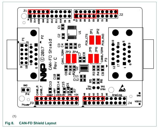
The CAN-FD Shield has a double-height DB9 connector installed by default (P3) for CAN/CAN-FD connections.
