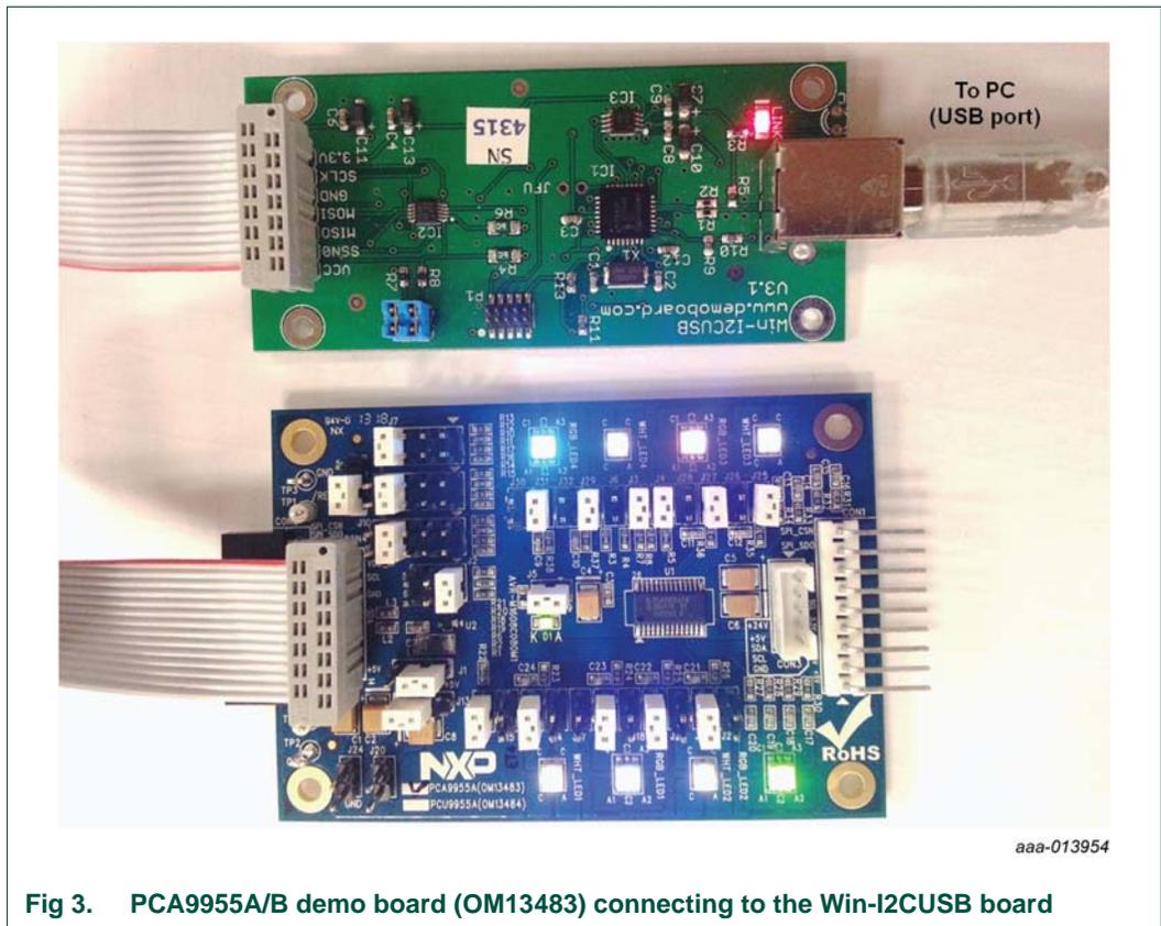
**Fig 3. PCA9955A/B demo board (OM13483) connecting to the Win-I2CUSB board**
