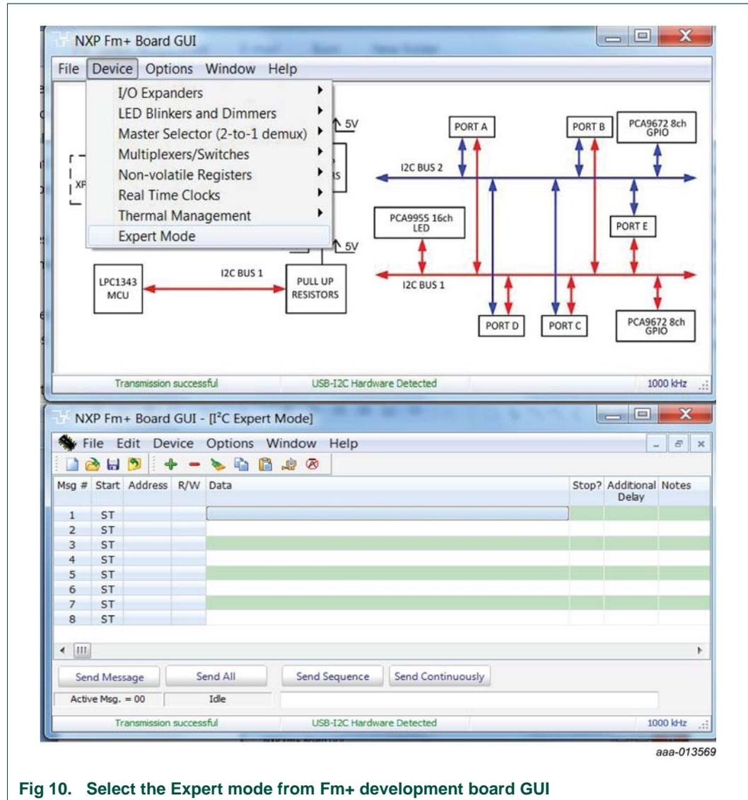
**Fig 10. Select the Expert mode from Fm+ development board GUI**
