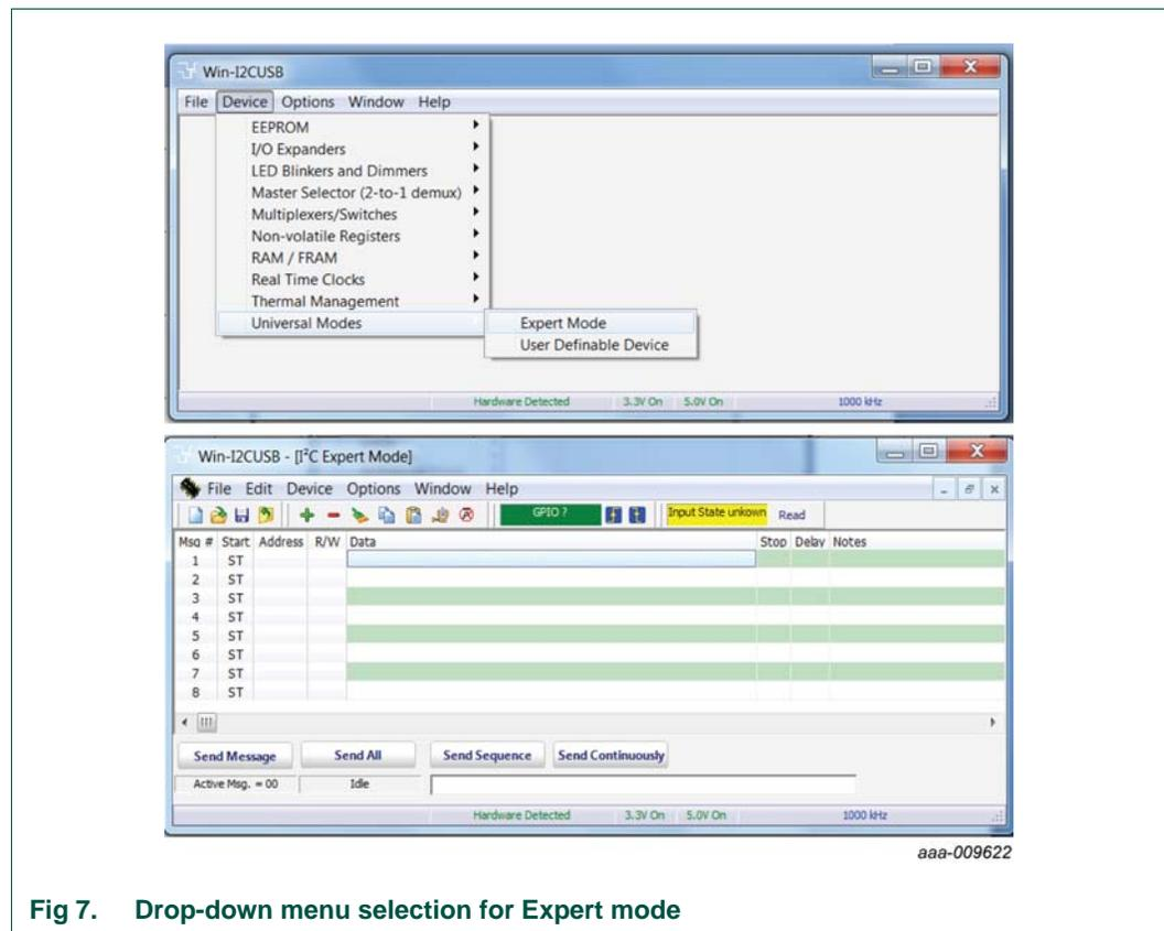
Fig 7. Drop-down menu selection for Expert mode
