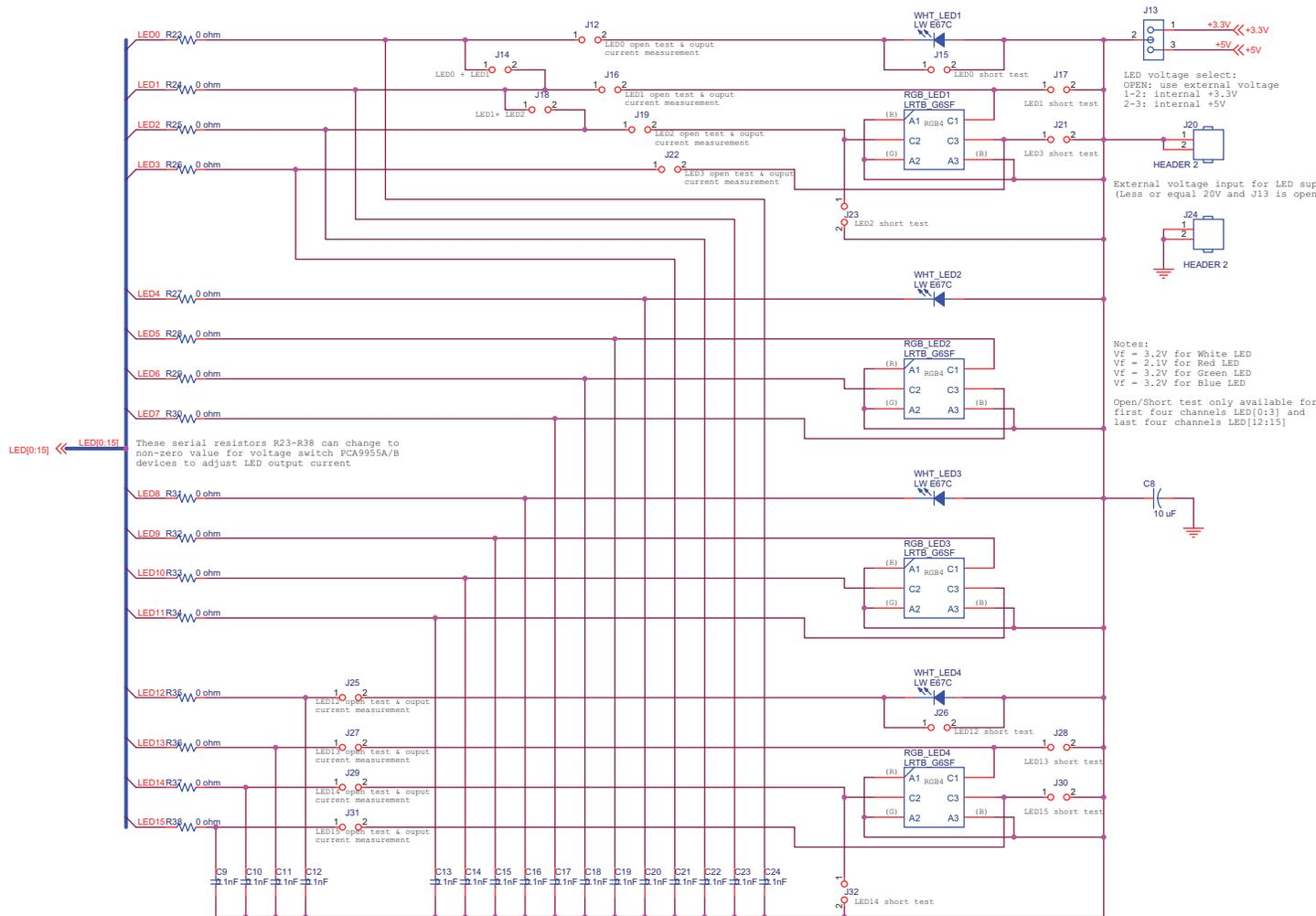
Fig 6. PCA9955A/B demo board schematic (part B)
