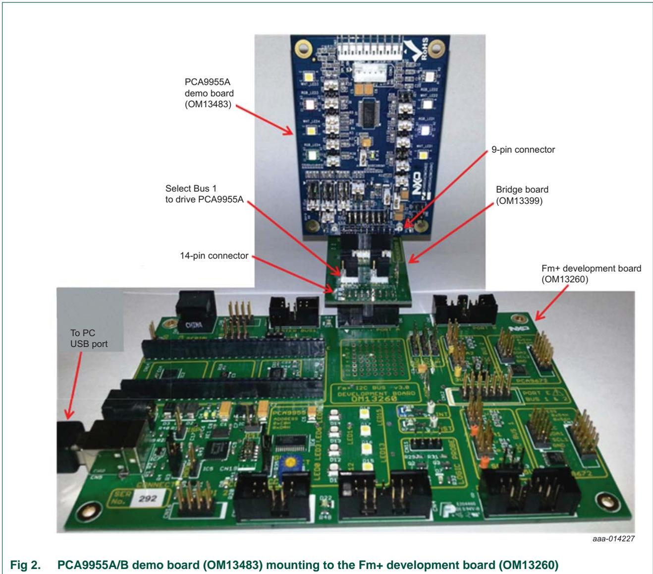
Fig 2. PCA9955A/B demo board (OM13483) mounting to the Fm+ development board (OM13260)
