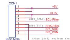
5-pin male connector to/from bus controller PCU9669 mini board to drive PCA9955A/B
