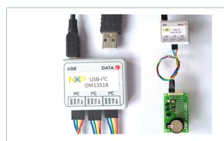
Fig 4. A) Dongle OM13518, B) connected to the evaluation board OM13514
