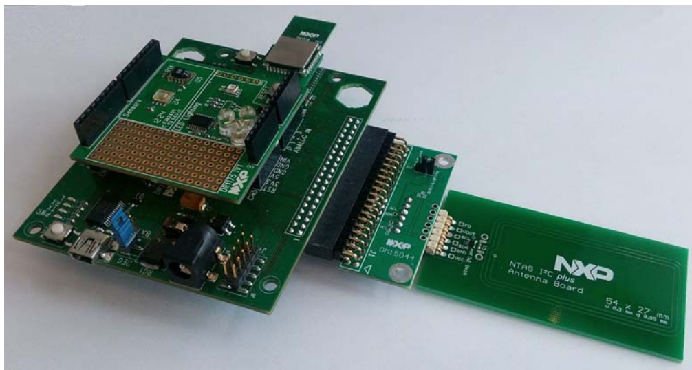
Figure 32: Fully Assembled Board with NFC Tag
