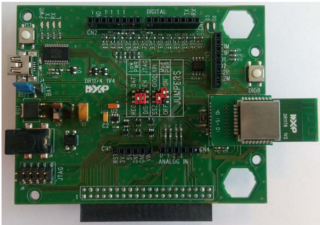
Figure 16: Carrier Board (with a JN516x Module)
