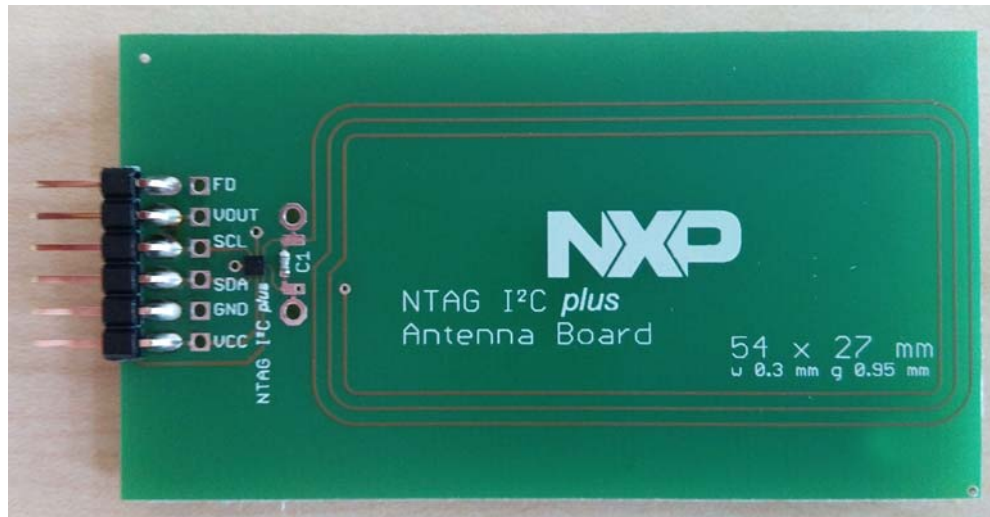
Figure 31: NTAG I 2 C plus Antenna Board
