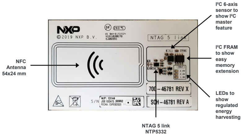
Front side of NTAG 5 link demo board
