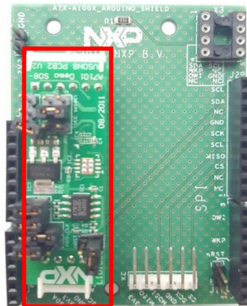
Fig 2. OM3710/A71CHPCB board mounted into the Arduino interface board
