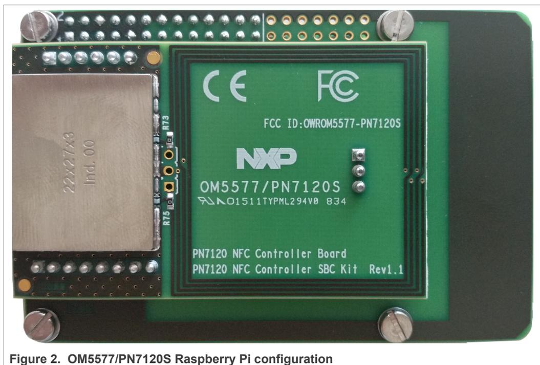
Then stacked together the boards with the Raspberry Pi according to below guidelines.
