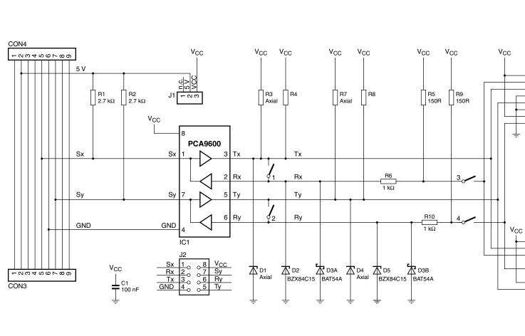
Fig 1. OM6293 PCA9600 evaluation board
