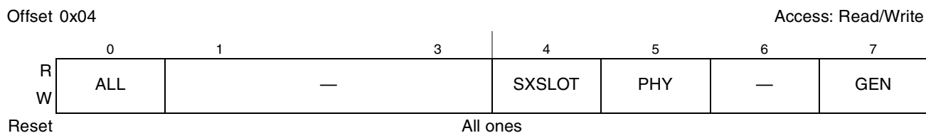
Figure 30. Reset Control Register (PX_RST)
