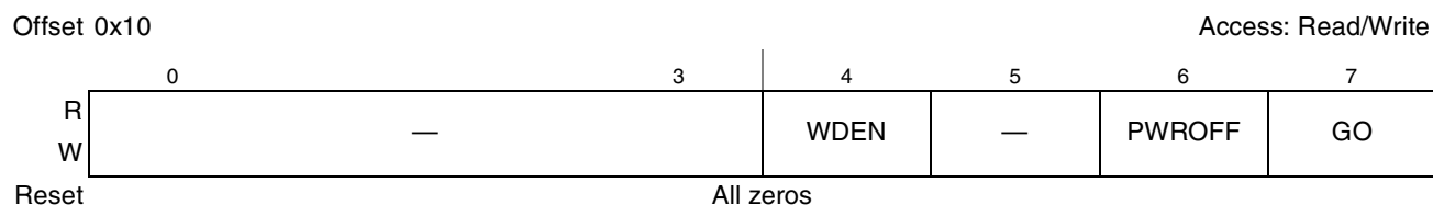
Figure 37. VELA Control Register (PX_VCTL)
