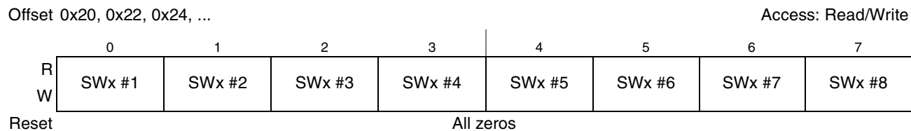
Figure 44. Switch Registers (PX_SWx)
