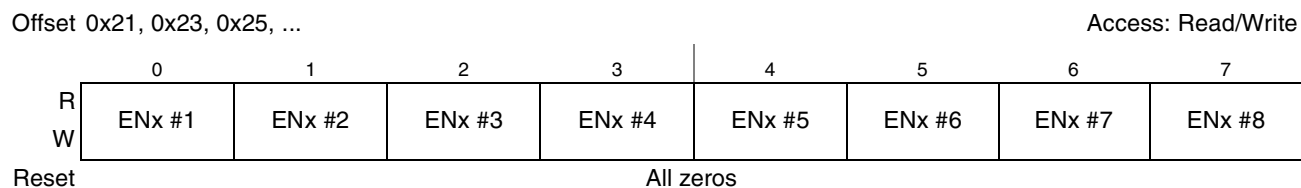
Figure 45. Switch Enable Register (PX_ENx)
