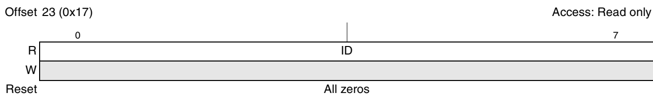
Figure 26. ID Register (PX_ID)
