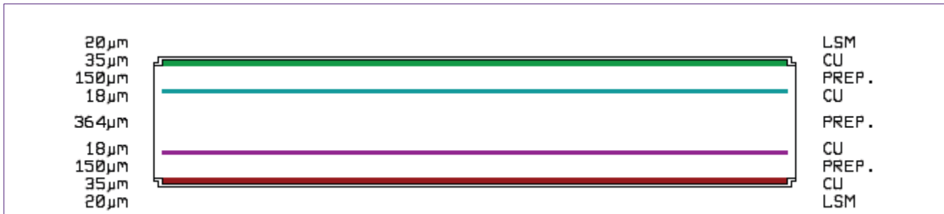
Fig 3. Layer stack of modified R_{th} -PCBs
