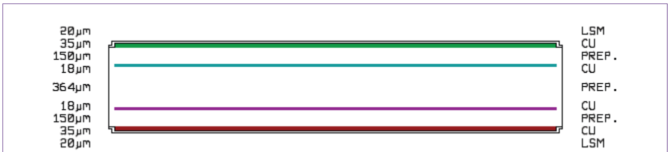
Fig 3. Layer stack of modified R_{th} -PCBs
