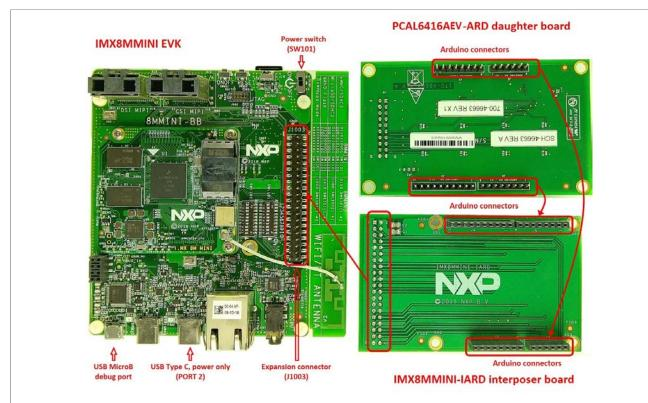
Figure 8. The assembly PCAL6416AEV-ARD daughter board, IMX8MMINI-IARD interposer board, and i.MX 8M Mini LPDDR4 EVK, before starting
