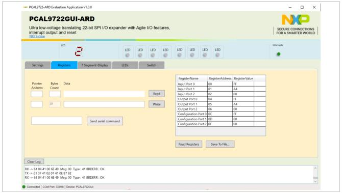
5. Use 7 Segment Display tab to run number up/down on display automatically, or select fix number to be shown on display.
