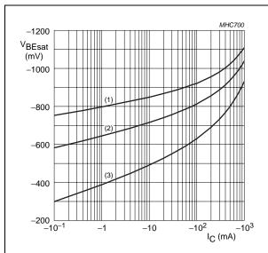
Transistor TR1;  $I_C/I_B = 20$ .
