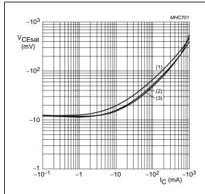
Transistor TR1;  $I_C/I_B = 20$ .
