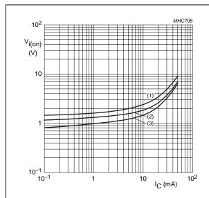
Transistor TR2;  $V_{CE}$  = 0.3 V.
