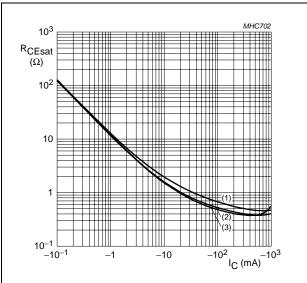
Transistor TR1;  $I_C/I_B = 20$ .
