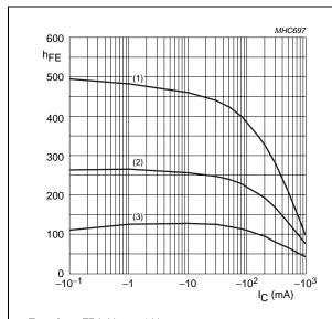
Transistor TR1;  $V_{CE}$  = -2~V.
