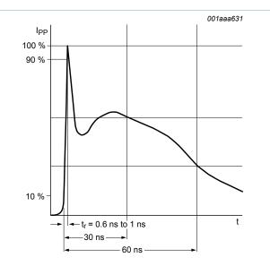
Fig. 2. ESD pulse waveform according to IEC 61000-4-2
