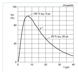
Fig. 1. 8/20 µs pulse waveform according to IEC 61000-4-5 and IEC 61643-321
