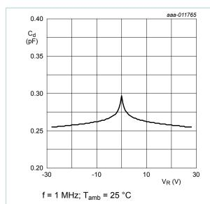
Diode capacitance as a function of reverse Fig. 3. voltage; typical values
