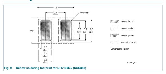
Ultra low capacitance bidirectional ESD protection diode
