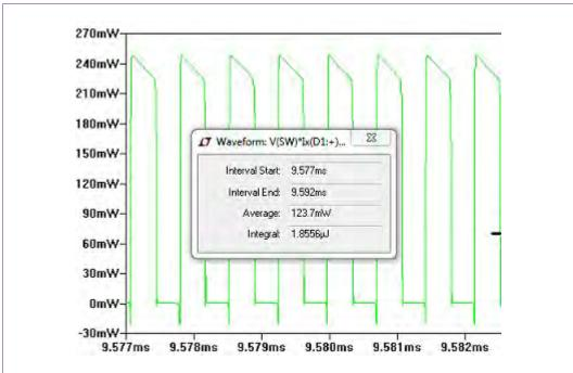
Fig 12. Power dissipation curve for a PMEG2005BELD with a 1 W white LED load and 2 V input voltage
