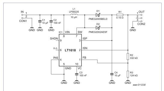
Fig 6. Schematic diagram of LED booster demo PCB with Schottky diode PMEG2005BELD (DFN1006D-2 / SOD882D) or PMEG2002AESF (DSN0603-2 / SOD962)
