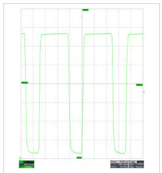
Fig 11. SPICE simulation of the switching node captured from the LED booster demo PCB for  $V_I$  = 2.5 V and a single 1 W white LED load.
