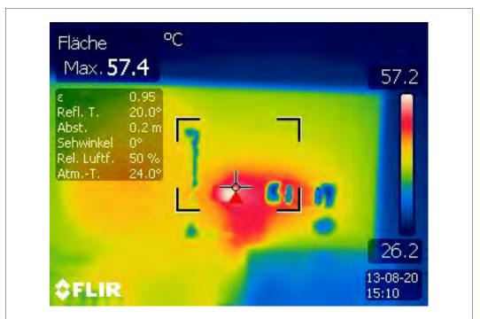
Fig 15. Infrared photograph of the LED booster PCB, area of the Schottky diode,  $V_I = 2 \text{ V}$ , load is 1 W white LED, with PMEG 2005BELD
