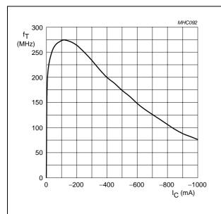
**PNP** transistor;  $V_{CE} = -10 \text{ V}$ .
