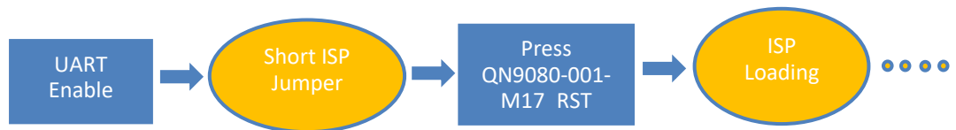
Fig 13. ISP download operation flow
