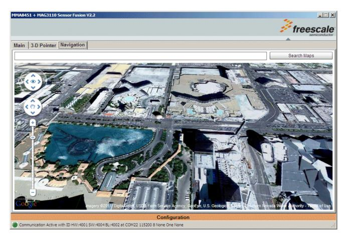
The Navigation screen uses all three angles output from the sensor daughter board to control the Google Maps display. The roll angle controls the display in the left and right direction. The pitch angle controls the display in forward and backward direction. The compass/yaw angle controls the rotation of the map display.
