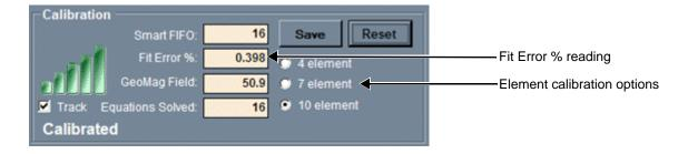
— Sequentially select the 10 element, 7 element, and 4 element option buttons.
