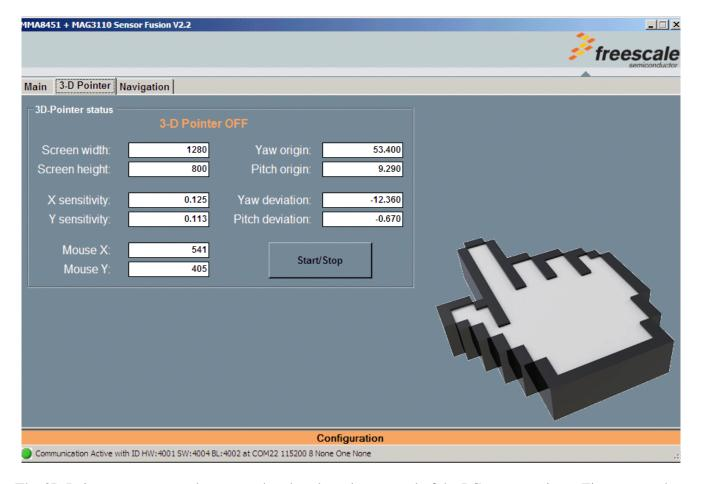
The 3D Pointer screen uses the sensor daughter board to control of the PC mouse pointer. First ensure that the compass is calibrated. To start the demonstration, click the Start/Stop button. The compass (yaw) and pitch angles are used to position the mouse pointer horizontally and vertically, respectively.
