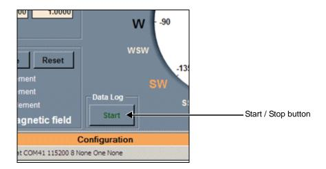
When the Start button is clicked, the user is prompted for the output filename and location. Because the file is written in the ASCII format, a .txt filename extension should be used. The data is written at a fixed rate of 10 Hz, irrespective of the sampling rate selected for the eCompass.
