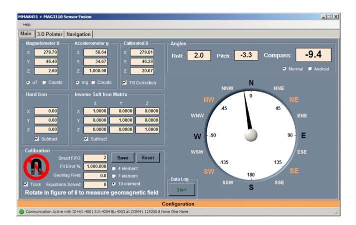
2. Rotate the device in a figure-eight motion as advised.
