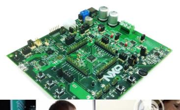
General Purpose S12 MagniV 16bit MCU with 5V and 3.3V voltage regulator with LIN-physical layer
