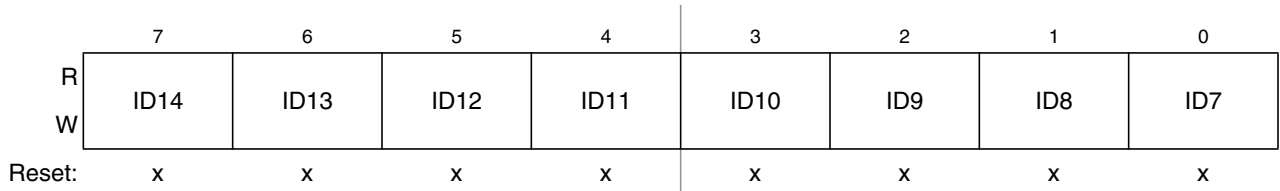
Figure 16-28. Identifier Register 2 (IDR2) — Extended Identifier Mapping
