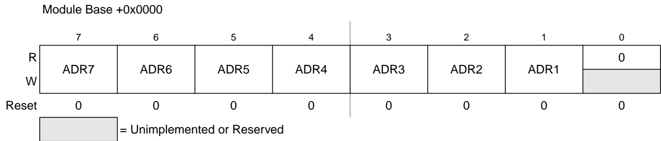
Figure 12-3. IIC Bus Address Register (IBAD)
