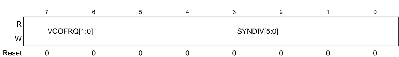
Figure 7-3. S12XECRG Synthesizer Register (SYNR)
