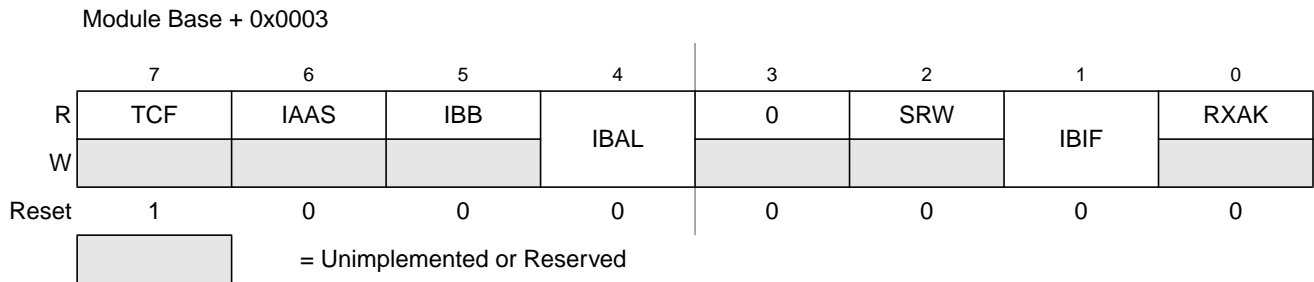
Figure 12-7. IIC Bus Status Register (IBSR)
