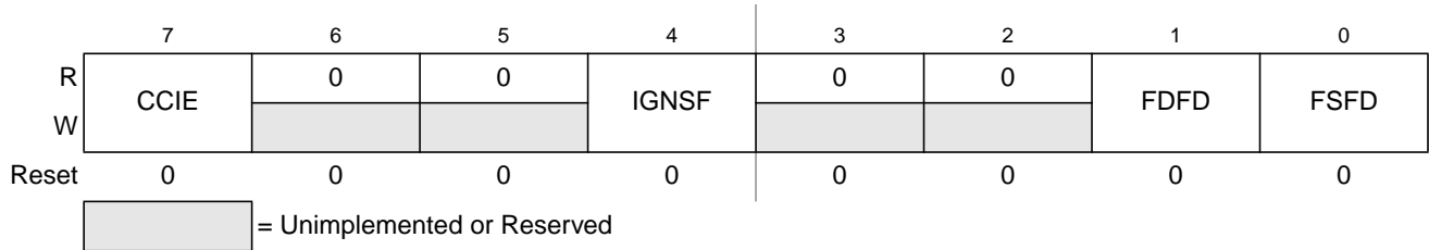
Figure 19-9. Flash Configuration Register (FCNFG)
