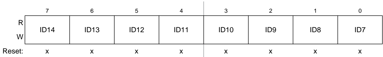
Figure 11-28. Identifier Register 2 (IDR2) — Extended Identifier Mapping
