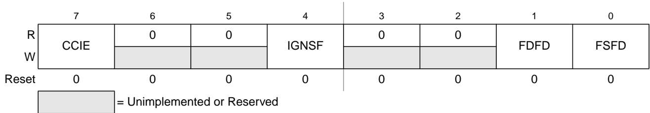
Figure 18-9. Flash Configuration Register (FCNFG)
