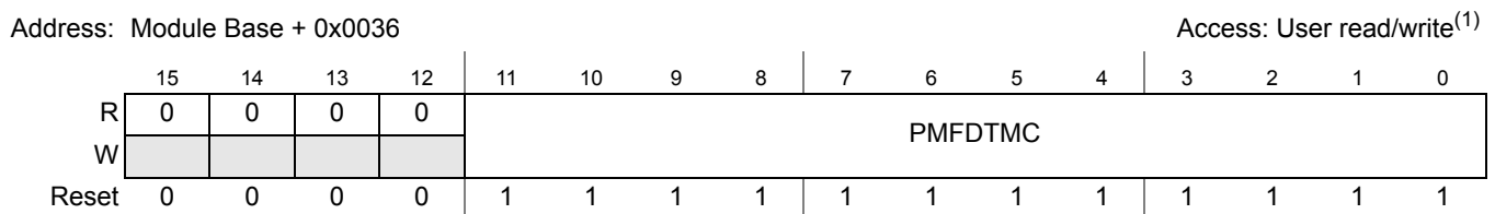
Figure 15-38. PMF Deadtime C Register (PMFDTMC)
