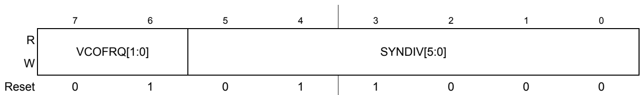
Figure 8-9. S12CPMU_UHV_V10_V6 Synthesizer Register (CPMUSYNR)
