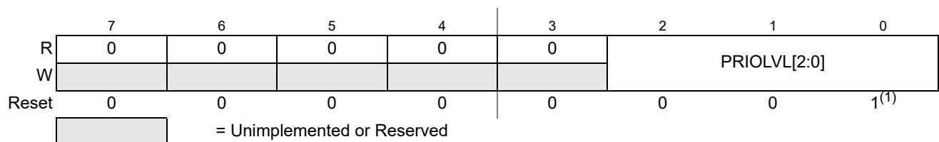
Figure 4-6. Interrupt Request Configuration Data Register 1 (INT_CFDATA1)
