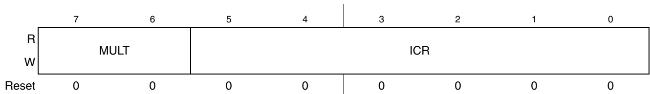
Figure 11-4. IIC Frequency Divider Register (IICF)
