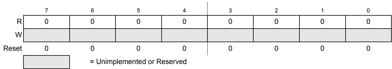
Figure 28-19. Flash Reserved2 Register (FRSV2)
