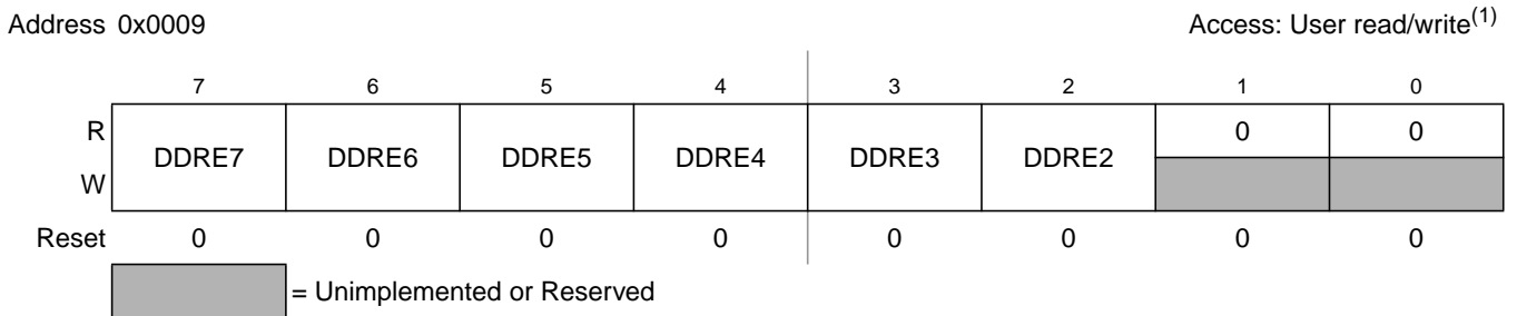
Figure 2-7. Port E Data Direction Register (DDRE)
