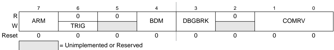
Figure 6-3. Debug Control Register (DBGC1)
