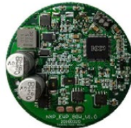
S12ZVM-EWP Electrical Water Pump S12ZVML64 reference design
