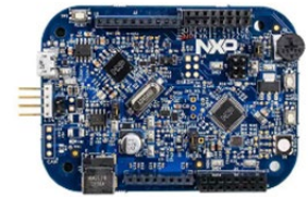
DEVKIT-S12ZVL LIN node S12ZVL32 evaluation board
