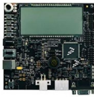
TRK-S12ZVHY64 Instrument cluster S12ZVHY64 evaluation board
