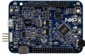
DEVKIT-S12ZVC CAN node S12ZVC192 evaluation board
