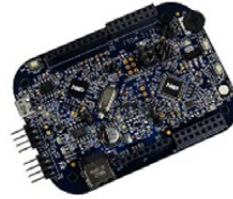
DEVKIT-ZVL128 LIN node S12ZVL128 evaluation board
