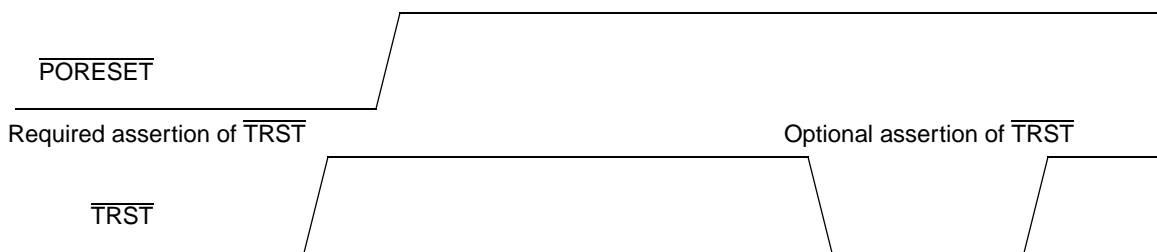
Figure 62. \overline{\text{PORESET}} vs. \overline{\text{TRST}}
