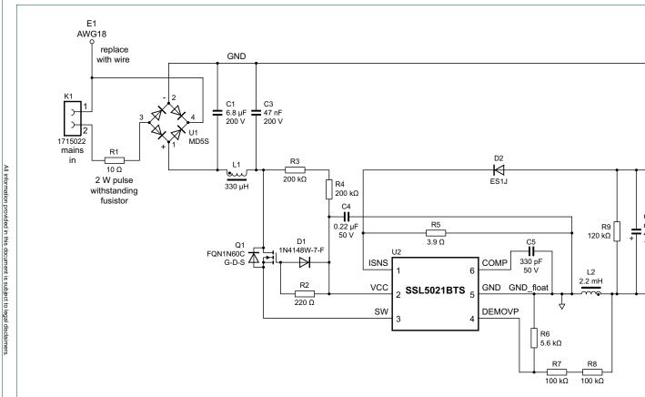
Fig 11. SSL5021BDB1205 demo board schematic
