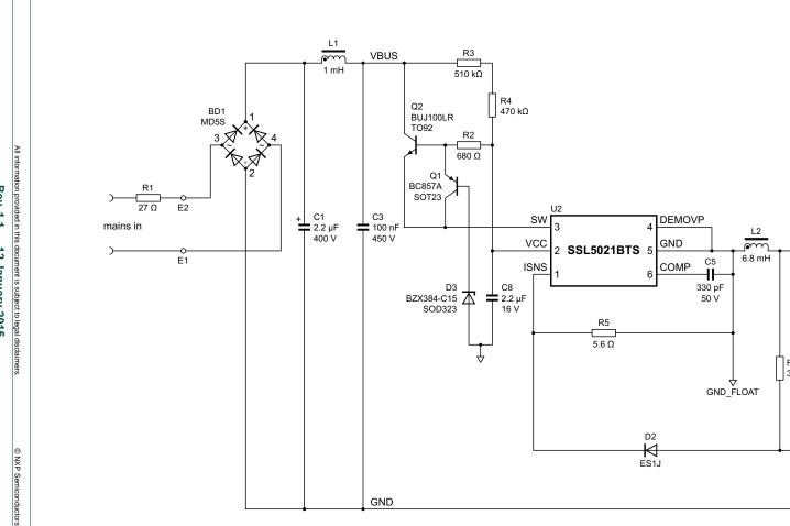
Fig 11. SSL5021BDB1267 demo board schematic diagram
