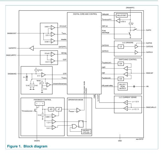
Digital controller for high-efficiency resonant power supply
