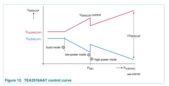
When the output power (P<sub>out</sub>) is at its maximum, the low capacitor voltage level (V<sub>Is(SNSCAP)</sub>) is at its minimum and the high capacitor voltage (V<sub>hs(SNSCAP)</sub>) is at its maximum level. According to Equation 1 in Section 8.2, the maximum  $\Delta V_{SNSCAP}$  (V<sub>hs(SNSCAP)</sub> – V<sub>Is(SNSCAP)</sub>), which is the divided  $\Delta V_{Cr}$  voltage, corresponds to the maximum output power.
