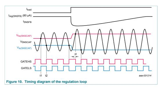
When the divided resonant capacitor voltage ( $V_{SNSCAP}$ ) exceeds the capacitor voltage high level ( $V_{hs(SNSCAP)}$ ), the high-side MOSFET is switched off (see Figure 10 (t1)). After a short delay, the low-side MOSFET is switched on. Because of the resonant current, the resonant capacitor voltage initially increases further but eventually drops.
