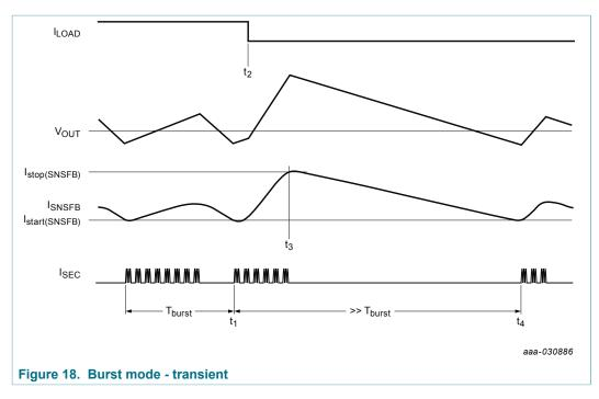
At t1, the system starts with a new burst cycle period. Shortly later at t2, the output load is reduced. As a result the output voltage shows an overshoot and the optocoupler current increases. To limit the overshoot, the system also ends the burst cycle when the optocoupler current exceeds the  $I_{stop(burst)}$  level.
