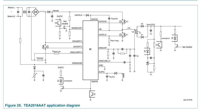
Digital controller for high-efficiency resonant power supply
